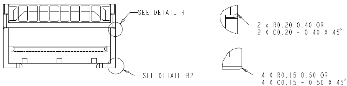
Figure 3-5: OSFP corner radius
